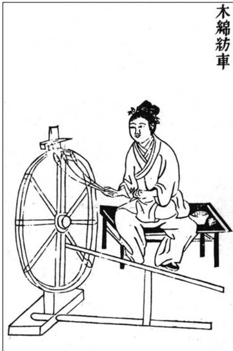
Agriculture in China. Fig. 6 Spinning wheel for making cotton yarn. When Wang Zhen was writing in the early fourteenth century, cotton was just beginning to replace other vegetable fibers as the most common everyday cloth, and Wang provides copious documentation about the techniques and equipment involved. Nongshu 25/6b.
